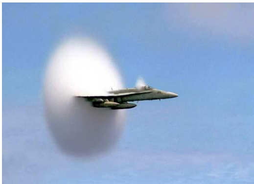
An F/A-18 Hornet passing through the sound barrier: A combination of conditions (water vapor, density and temperature) must occur to create this event.
